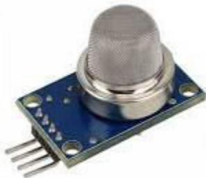
The MQ-6 module is used in gas leakage detecting equipment in family and industry, This module has high sensitivity to LPG, iso-butane, propane and LNG. It can also be used to detect the presence of alcohol, cooking fumes, and cigarette smoke. The module gives out the concentration of the gases as a analog voltage equivalent to the concentration of the gases. The
